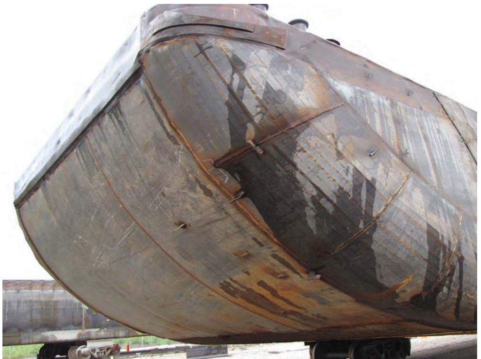
The 40-foot tandem ProForm press brake allows McGinnis to bend large pieces of A36 steel plate, including the head log - a heavily reinforced section at each end of a barge. "On many of these barges [the head log] is 30-foot long," said Rick Griffith, president, McGinnis. "We are one of very few shops on the river that can bend it in one piece."
